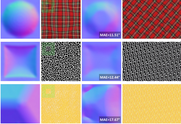
Figure 5: Shape and texture results for synthetic images. From left to right: surface normals of the true shape; input image; output surface normals (with MAE); and sample from output texture generator. Green inset squares show patch sizes used by the unwarper.
